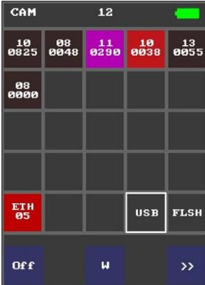
To enable or disable the mode of detecting USB cameras, briefly press the stylus or your finger on the “USB” cell, the “On” or “Off” checkbox will appear in the lower left corner of the screen.
