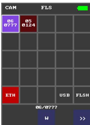
To move the cameras to the "white" list from the home screen, first touch the selected cell with your finger or stylus (it is highlighted with a white border), and then click on the "W" button – the cell with information automatically moves to the second page of the screen and turns green.
