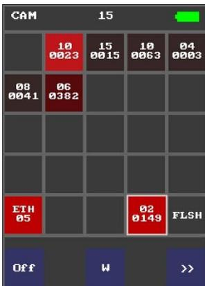
For searching and localizing the detected video camera press the cell and hold for two seconds, then a scale (column) with the signal level will appear on the screen.
