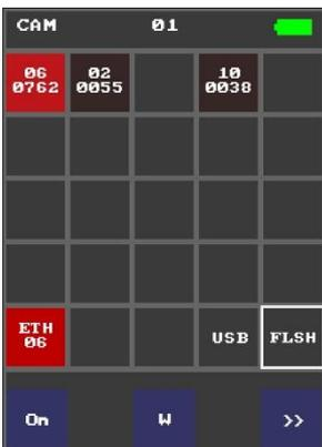
To search and localize the detected video camera press the cell and hold for two seconds, then a scale (column) with the signal level will appear on the screen.
