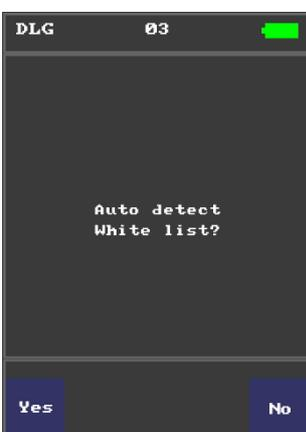
The device provides a mode for automatically transferring all currently detected signals to the "white" list. To do this, on the main screen, without selecting a specific cell, press the "W" button. You will be asked to start the automatic detection mode and transfer signals to the "white" list.
