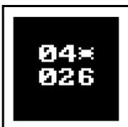
Information about detected video cameras and suspicious signals is displayed on the "main screen" of the device - there are "cells" with numbers (bin file) in the form of table cells, the fields of which are highlighted in shades of red (depending on the degree of probability of matching with the "images" of cameras) or lilac (when a line or frame pulses RDT is detected in the signal).
