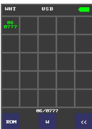
To do this, select a single cell (highlighted with a white border) and press the "ROM" button, you will be asked to write the information to the internal memory of the device. The stored cell will be displayed with the "\*" icon. Pressing the "W" button returns the information back to the home screen.
